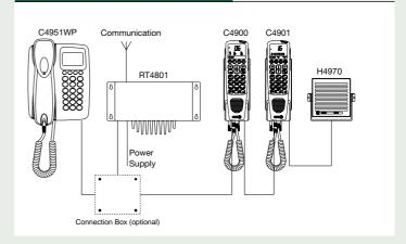
The SAILOR VHF RT4801 includes in a basic configuration a transceiver unit and a handset control unit. The units are connected by means of the SPARC-bus interface. This advanced balanced data and AF interface can be used to interconnect multiple control units as well as exterior computer based control/ programming options. The maximum distance between transceiver unit and handset control unit may be up to 40m in 12VDC installations, in 24 VDC installations up to 80m.
